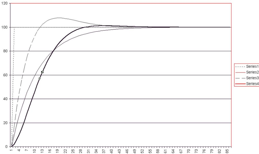
By marginally increasing the overshoot to about 2.3% by altering the feedback constant and changing the exponential constants to 18.2 to re-align the curve with the standard crossover at 80%, this response then even looks better.
